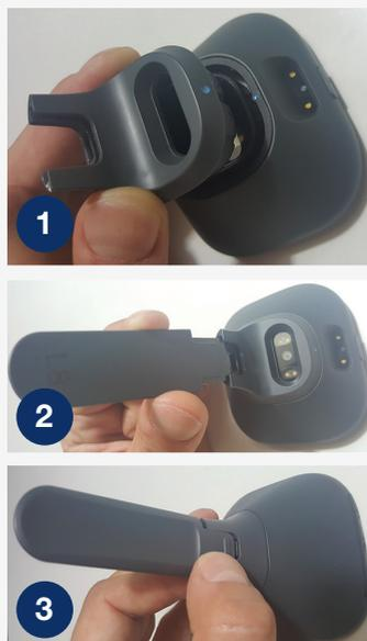
Figure 10 – Connecting the Tongue Depressor
